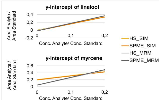
Figure 4: Corresponding calibration curves (in beer simulant) measurements of Fig. 3. Comparison of y-intercept of myrcene and linalool.
