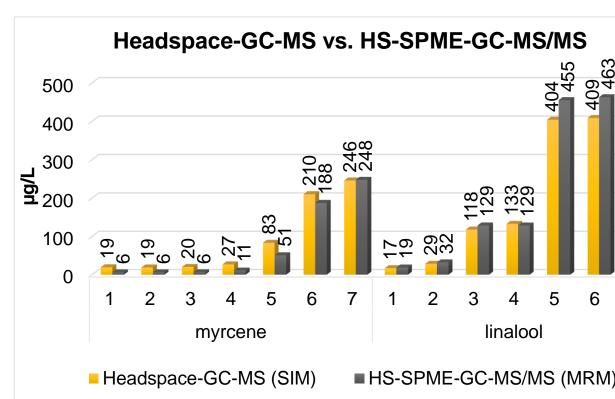
headspace-GC-MS method wit thod with 7 different beers. The samples are measured in duplicates (RSD < 10%).
