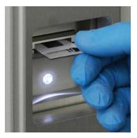
3. Insert chamber into instrument
