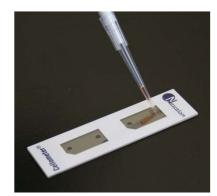
2. Pipette 20uL into counting chamber
