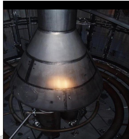
Cleaned with Alkaline + Hydrogen Peroxide (oxidizer)
