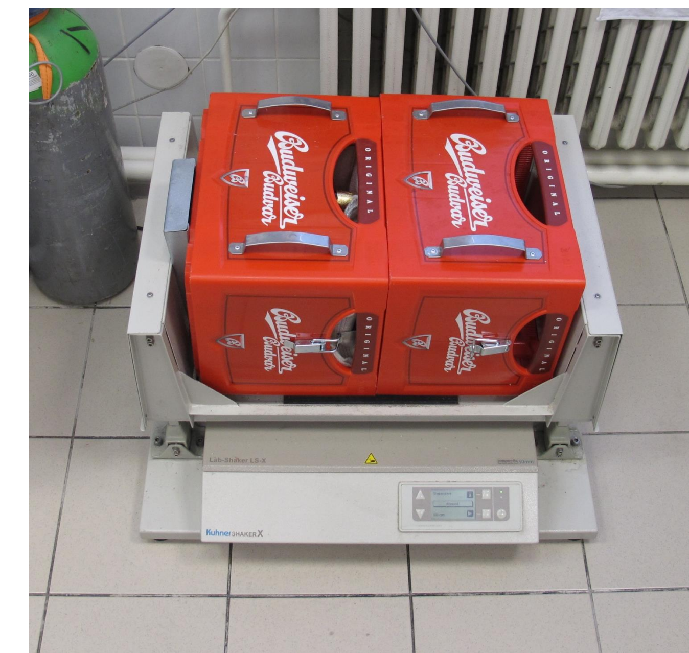
Fig. 2 Beer bottle shaker for two crates filled with bottles or cans.
