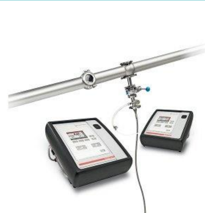
Figure 1. CBox hooked up to an in-line connection, as used in wort oxygenation
