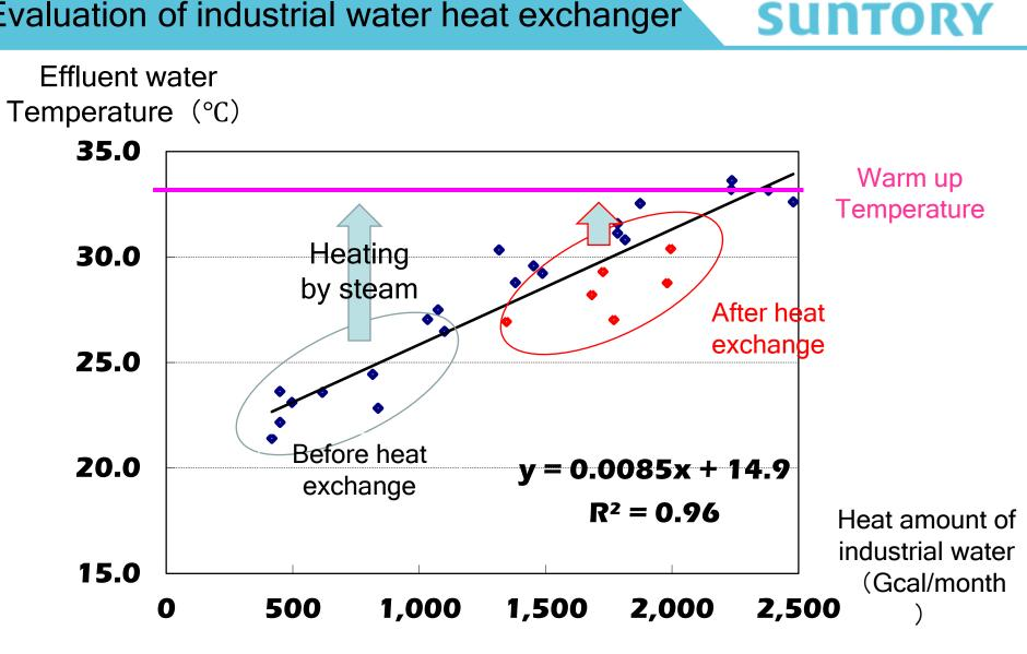
Correlation in the heat amount of Industrial water and Effluent water temperature
