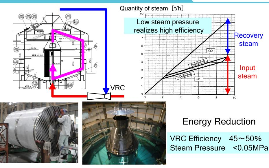
Re-designed the thermal compression and the internal boiler to run with lower steam pressure for higher heat recovery
