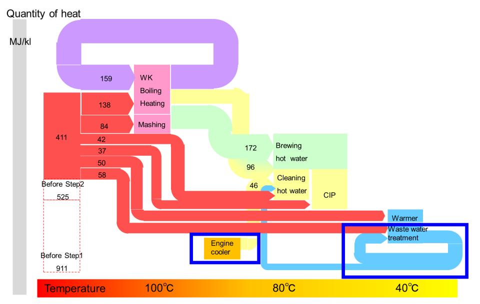
Increasing heat recovery from Trigeneration and Waste water treatment
