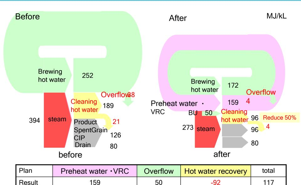
Increasing of heat recovery and Reduction of Overflow
