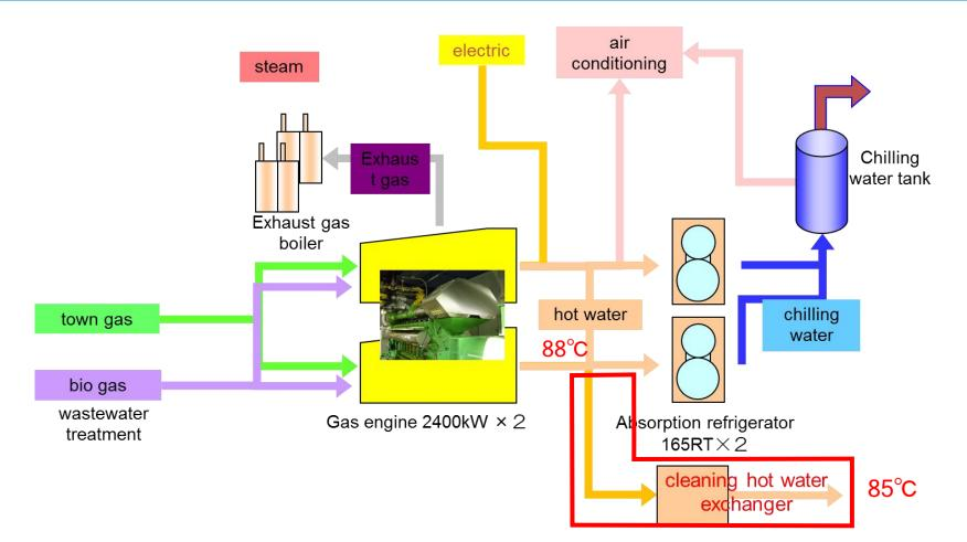
Exhaust heat of Trigeneration recovered by Cleaning hot water, which means water used at Clean-in-place
