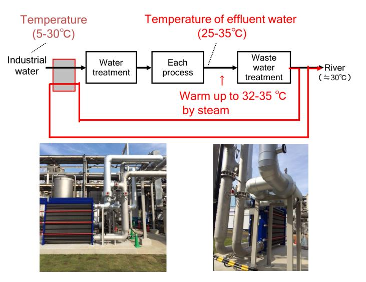
Reduction of Heating steam by heat exchanging between treated wastewater and industrial water
