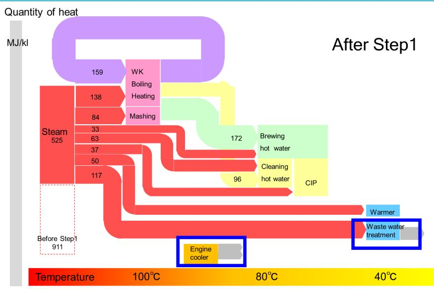
Optimized recovery of waste heat by heat exchange in sources with close temperature conditions in whole plant
