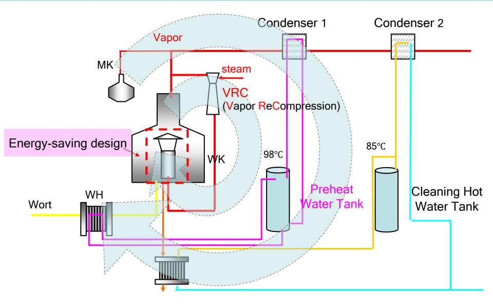
Installation of Closed 3-Loop Heat Recovery
