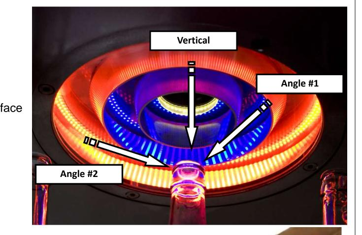
Multi-Angle finish inspection helps prevent bottle break on pry-off
