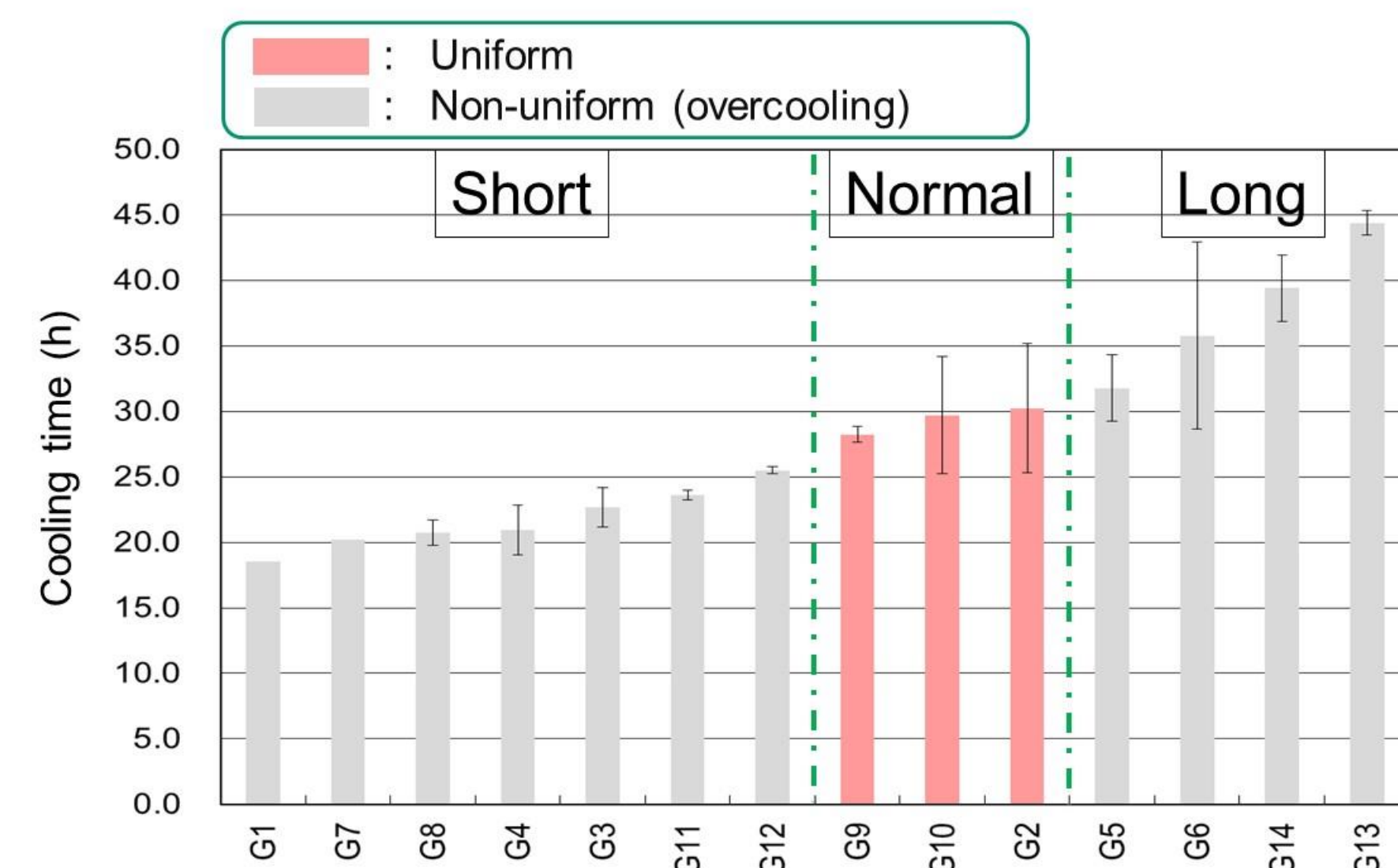
Fig.3 Variation in cooling time in individual tanks To classify the patterns of cooling and temperature distribution, coolant flow rate was measured (Fig. 4). If the ratio of coolant flow rate between cylindrical and conical regions was not well balanced, overcooling occurred (Fig.4, Short and Long). Maintaining the appropriate ratio of flow rate is critical for uniformity of temperature distribution.
