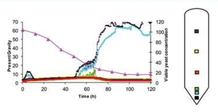
Figure 1. Actual measurements of viable yeast concentrations throughout a CCT during the course of a conventional (unmixed) fermentation, clearly illustrating the premature settling of yeast in the cone of the tank.
