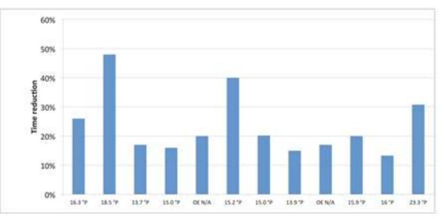
Figure 3. Process time reductions for dynamic fermentation. Results for 11 different breweries and 12 different brands, including OE for each case, when known.
