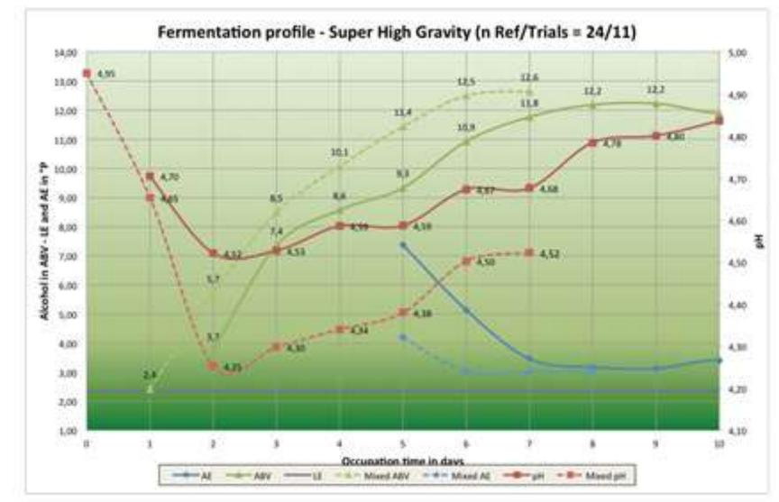
Figure 5. Fermentation profiles for Dynamic vs. Standard fermentation of VHG beer (OE=24.5°P), showing the differences in extract, alcohol and pH trends
