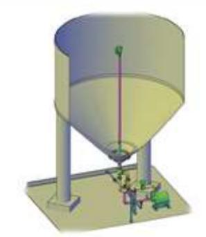
Figure 2. Dynamic fermentation system utilizing rotary jet mixing with bottom-entry installation. Liquid is circulated from the tank outlet through a centrifugal pump to the mixer, which distributes the incoming liquid to all areas of the tank. The system is installed through the tank swing cone and bottom outlet flange, minimizing necessary tank modification.
