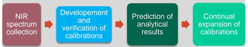
Calibrations were developed follow the steps above using the software from the instrument manufacture. Various combinations in wavelength selection and treatments, and mathematical models were used to achieve better accuracy and repeatability.
