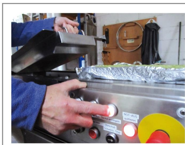
Open Chamber by Pressing Button and Pulling Handle at a Time
