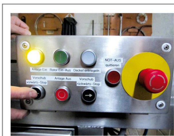
Press "Feed FORWARD - STOP"
