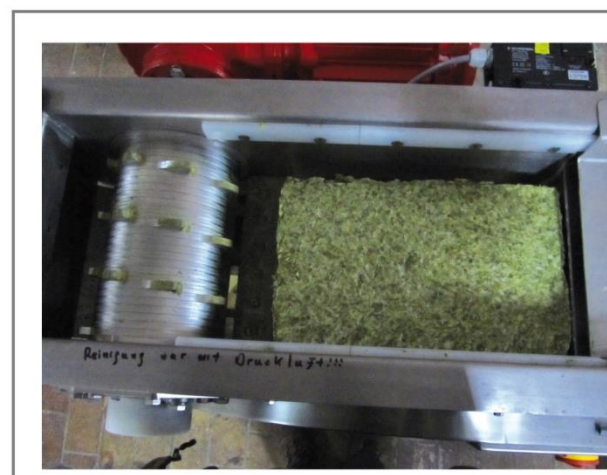
Insert Hop Block into Disintegration Chamber
