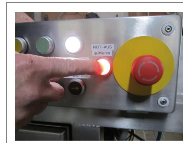
Press "Emergency Stop" to Revoke Safety Interlock
