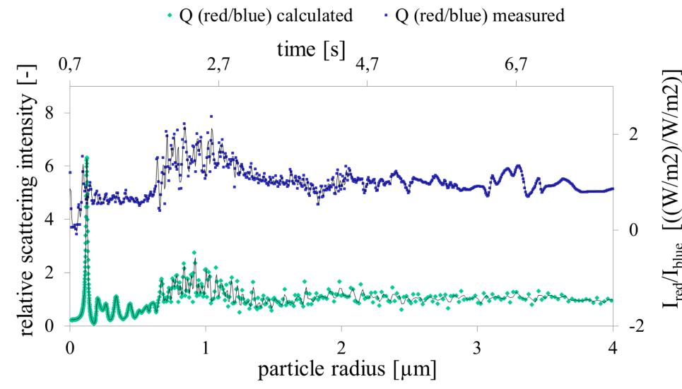
FIG.4: Comparison between measurement and simulation of solved and
