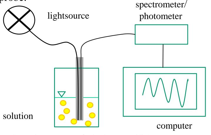
FIG.1: Laboratory setup for back scattered light measurement
