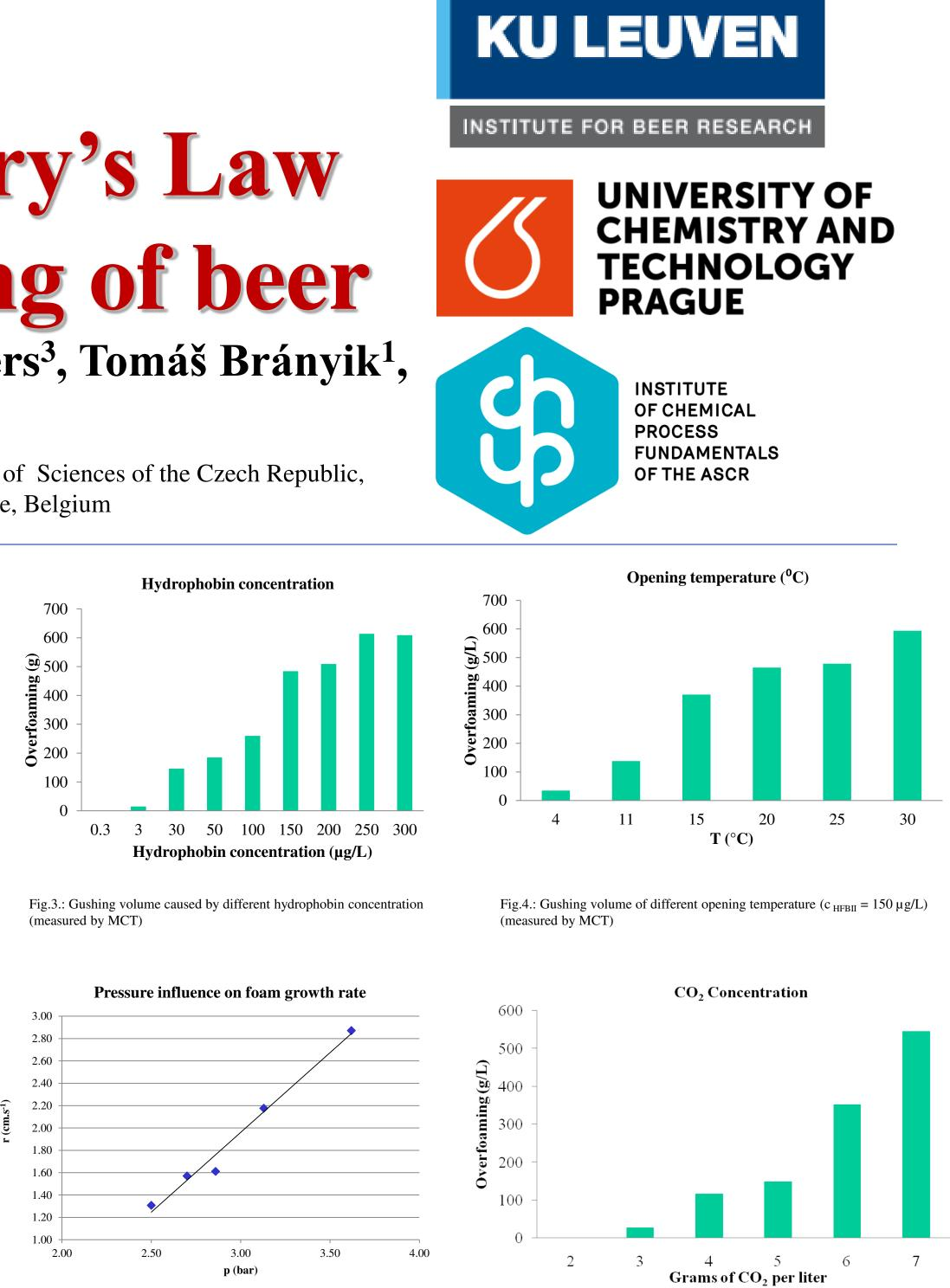
Fig.5.: Gushing foam growth rate characteristic of different pressure level (measured by DC): the intensity of foaming is directly proportional to the pressure used for the saturation of the solution. The maximum tested pressure (3.8 bar) was limited by the apparatus (DC).
