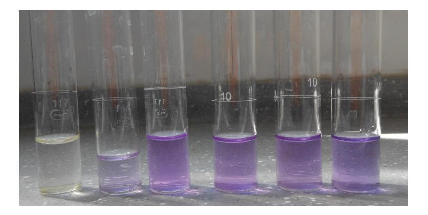
Anti–2,2-diphenyl-1-picrylhydrazyl (DPPH) radical capacity
