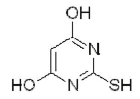
Thiobarbituric acid can react with carbonyl compounds in beer to generate a substance of yellow.At 530nm wavelength, they have specific absorption value. The lower value is, the more fresh beer is.
