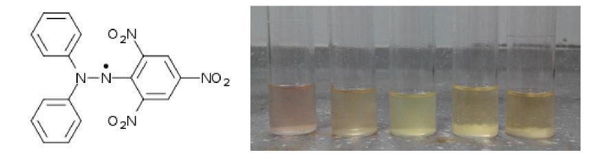
The radical scavenging capacities of beers were measured based on their ability to quench the DPPH radical, decrease the absorbance of DPPH radical at 515 nm.
