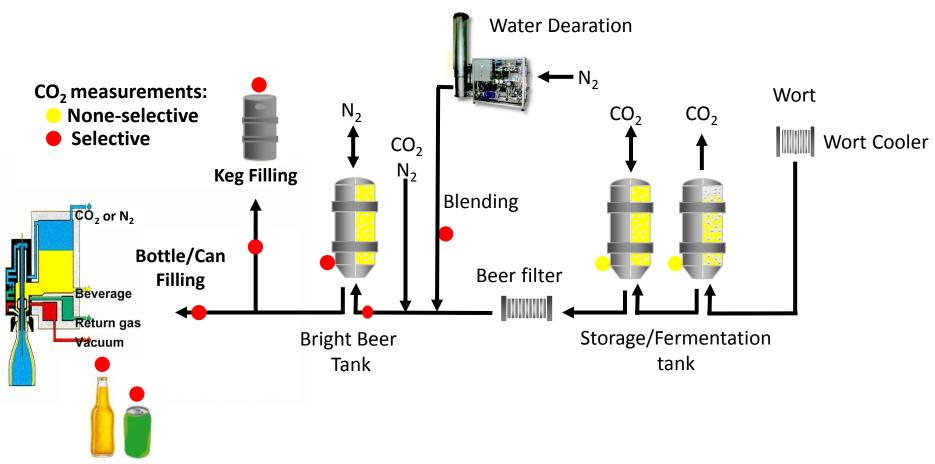
Medium used to transport beer, flush production lines and used as counter pressure on tanks is important in the choice of the CO<sub>2</sub> measurement.
