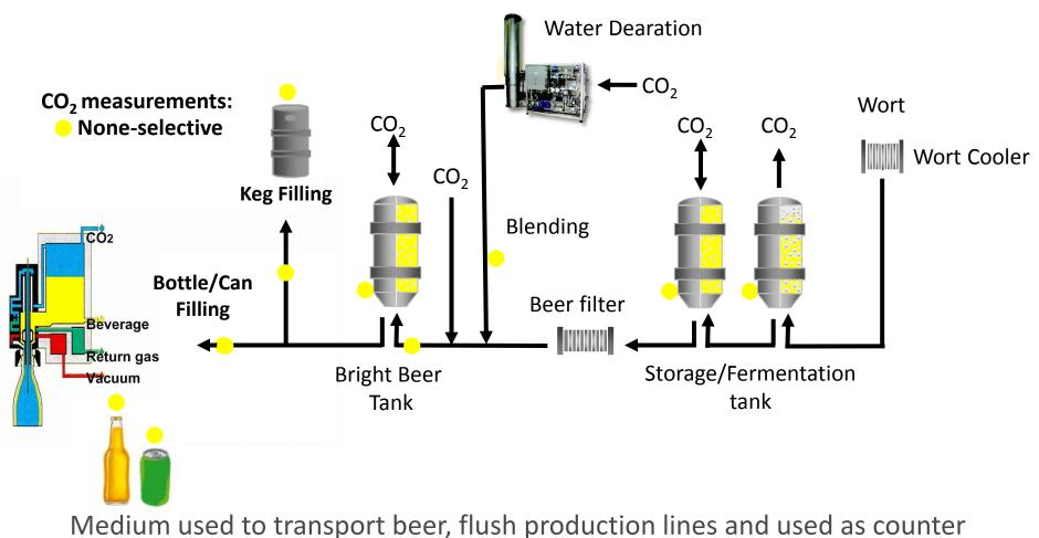
pressure on tanks is important in the choice of the CO<sub>2</sub> measurement.
