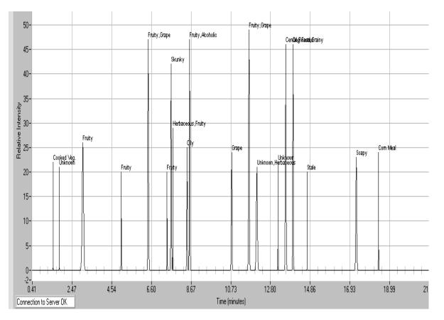
Serially dilute a sample and analyze by GC-MS with Olfactometry. The compounds that persist by olfactometry at the highest dilution levels can have the highest impact.
