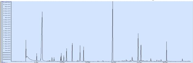
By selecting specific mass to charge ions for the analytes of interest, there is a sensitivity gain and minimal interference.
