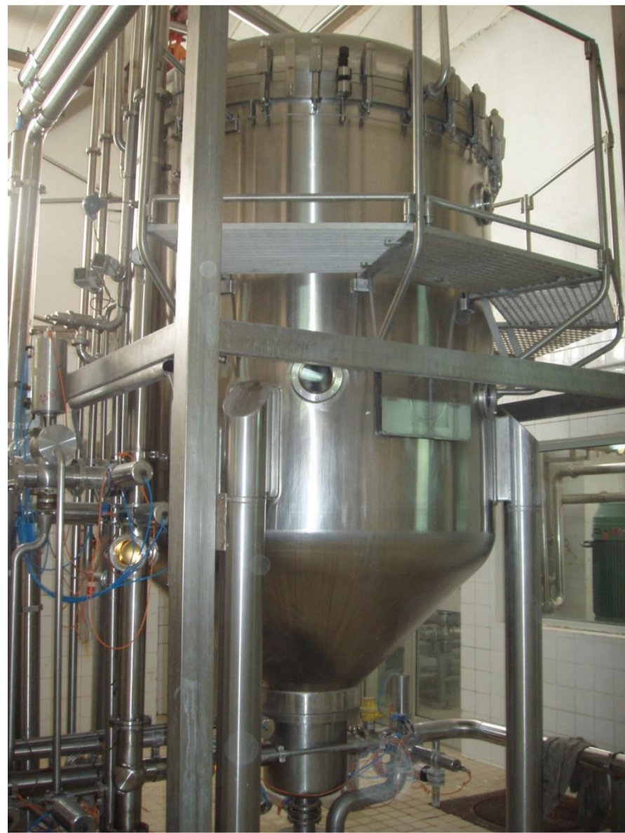
Filtrix candle filter (80m 2 ) with DE free single pre-coat of 770g/m 2 .
