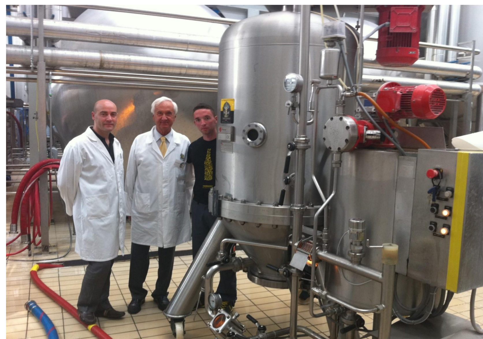
Horizontal plate filter (20m 2 ) with DE free single pre-coat and bodyfeed in Birra Theresianer.
