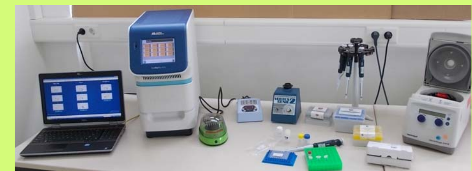
Minimum instrumentation and bench space needed to do PCR analysis
