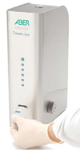
Figure 1 Countstar machine with slide being inserted into port.
