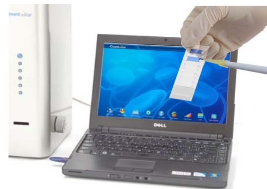
Figure 2 Countstar, software and dongle shown. Top right image of disposable 5 chamber slide with sample.
