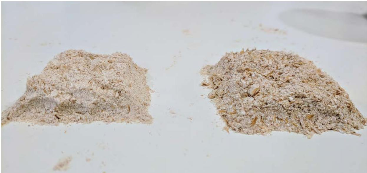
This figure shows the difference of appearance between the fine powder created when cleaning the chamber (left) and what the course flour used for evaluation in the method looks like (right).
