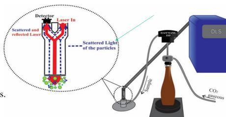
A specially designed dynamic light scattering (DLS) equipped with a sampling device capable of holding the sample under pressure at all times during analysis.
