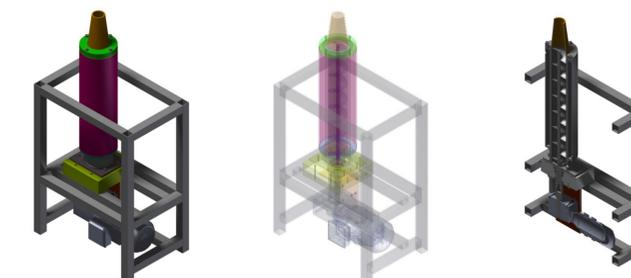
Plant design of a scrape chiller with pressing section
