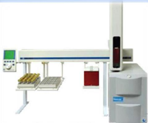
The Flash GC Nose system can analyze about two hundred aromatic compounds using two columns of different polarities in parallel
