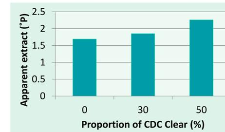
Figure 2. Last runnings using CDC Clear in a lauter tun
