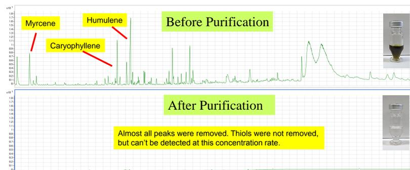
Figure 1. Total ion chromatogram of Hallertauer Tradition hop extract before or after solid-phase extraction with silver ion fixed SPE cartridge. Both extracts were ten times concentrated.
