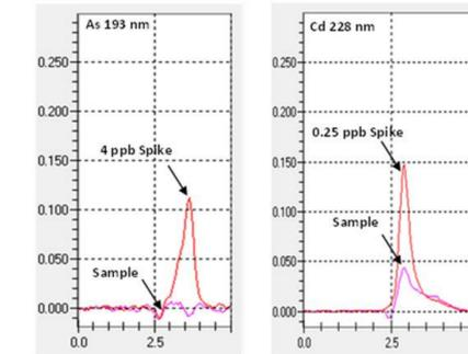
Fig 6: Arsenic & Cadmium Sample and Spike
