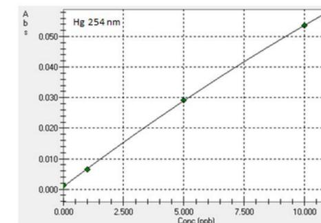
Fig 5: Mercury Calibration Curve
