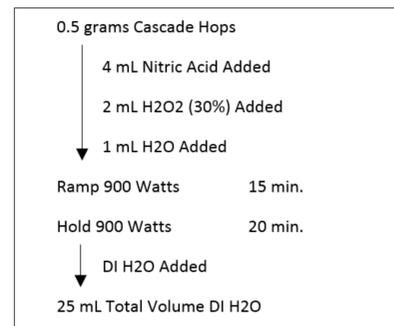
Fig. 1: Digestion/Preparation Procedure
