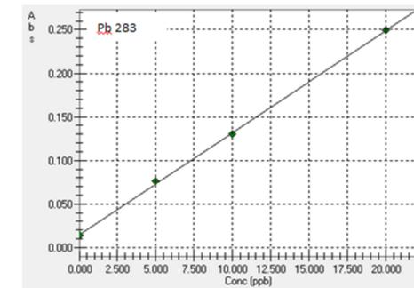
Fig 4: Lead Calibration Curve
