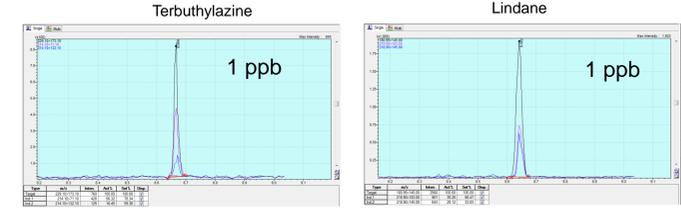
Figure 6 Example of Overlaid MRM Chromatograms For Two Pesticides in the 1-ppb Calibration Standard
