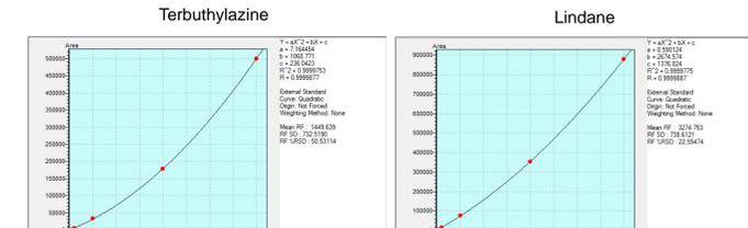
Figure 5 Exponential Calibration Curves for Two Pesticides, 1 to 200 ppb
