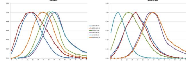
Figure 2: Optimized Transitions for Two Pesticides Using the MRM Optimization Tool
