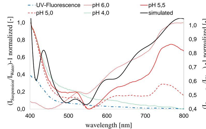
FIG.4: Comparison between measurement and simulation of solvated and precipitated gluten
