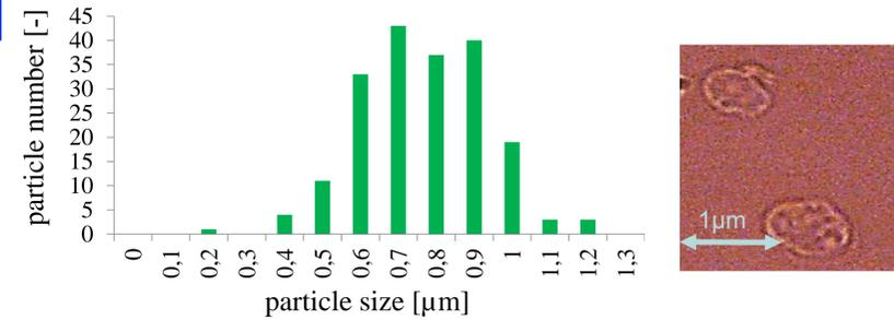
FIG.2: Particle size distribution of precipitated amino acids (left), proteins under a microscope (right)
