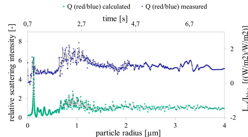
FIG.5: Measurement of calcium oxalate throughout precipitation reaction
