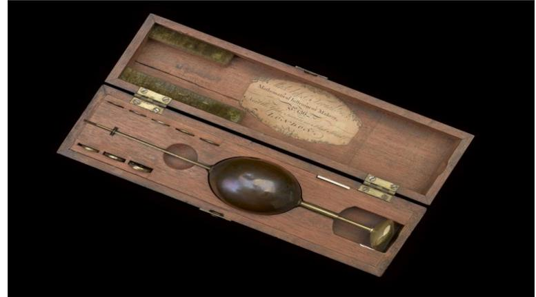
“Saccharometer” which allowed accurate measurement of wort strength
