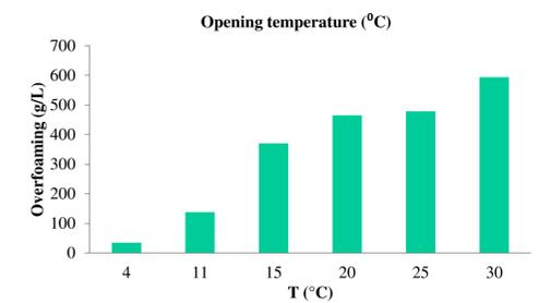
Fig.4.: Gushing volume of different opening temperature (c<sub>HFBII</sub> = 150 μg/L) (measured by MCT)
