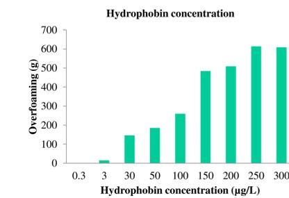
Fig.3.: Gushing volume caused by different hydrophobin concentration (measured by MCT)
