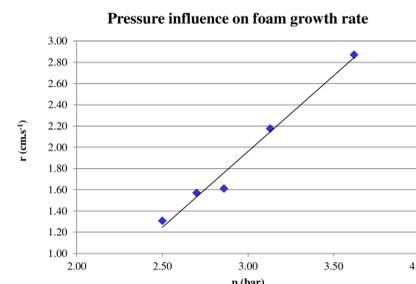
Fig.5.: Gushing foam growth rate characteristic of different pressure level (measured by DC): the intensity of foaming is directly proportional to the pressure used for the saturation of the solution. The maximum tested pressure (3.8 bar) was limited by the apparatus (DC).
