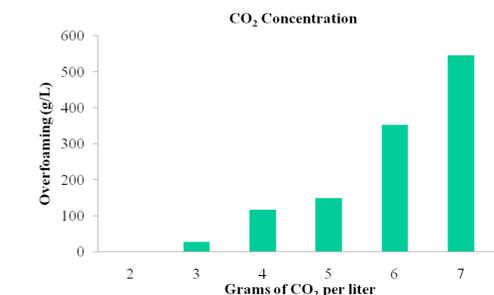
Fig.6.: Gushing volume of CO<sub>2</sub> content (c<sub>HFBII</sub> = 150 μg/L) (measured by MCT)
