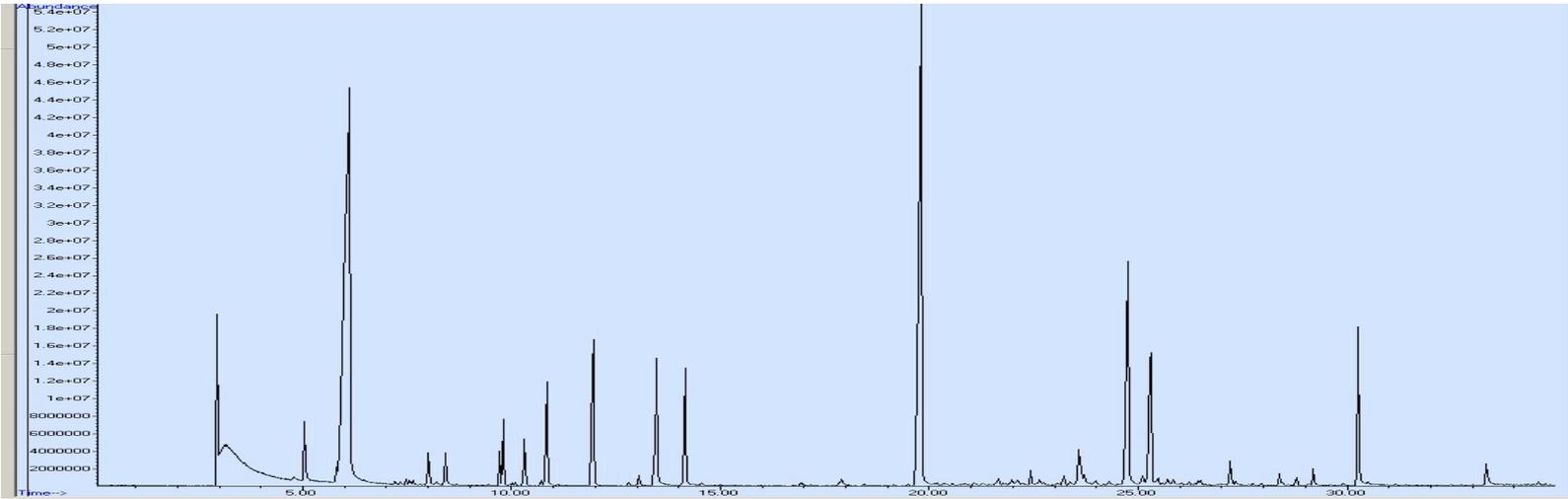
By selecting specific mass to charge ions for the analytes of interest, there is a sensitivity gain and minimal interference.
