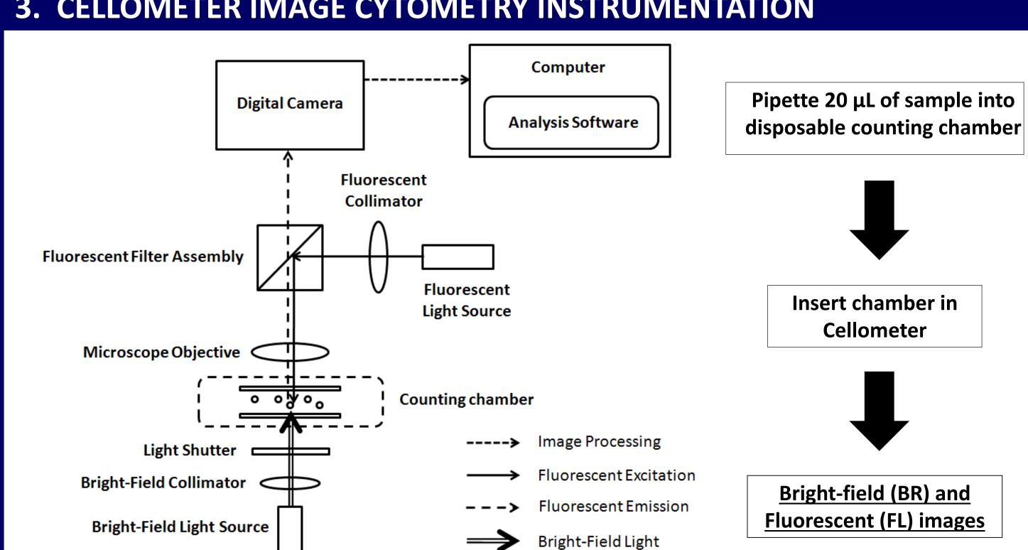
Cellometer image cytometer utilizes an epi-fluorescence setup for fluorescent image analysis
