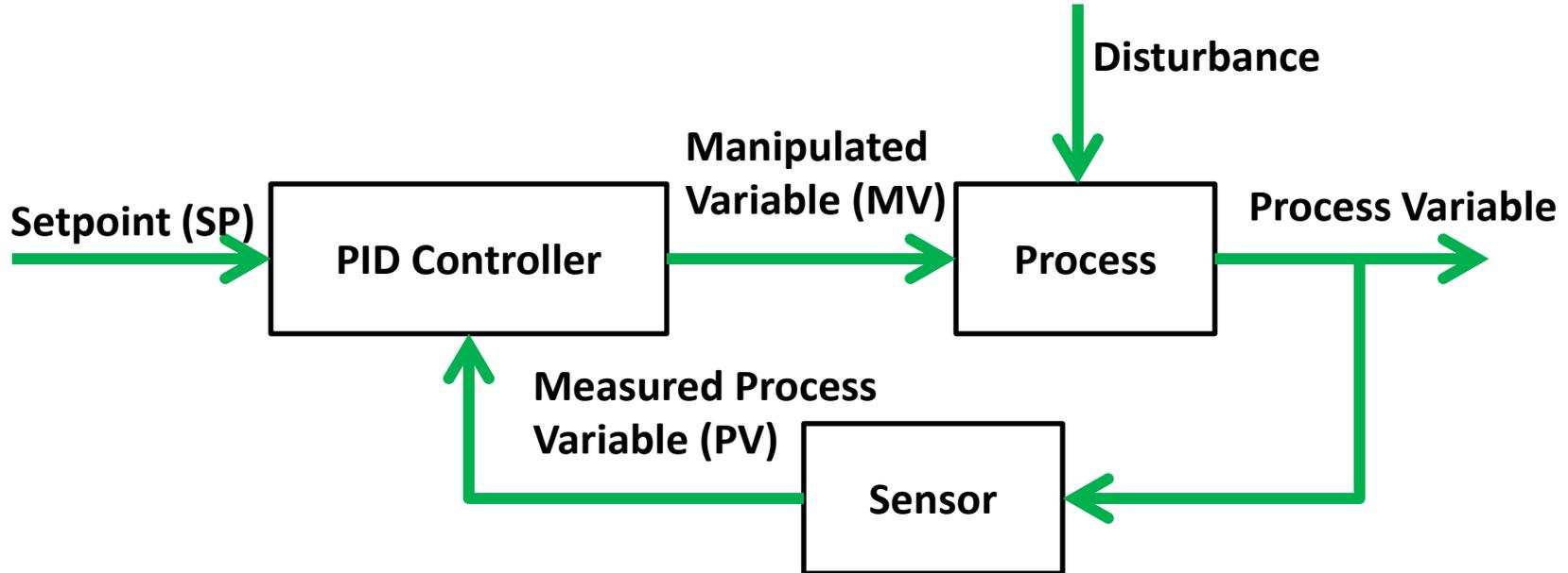
Classic block diagram of a PID Loop
