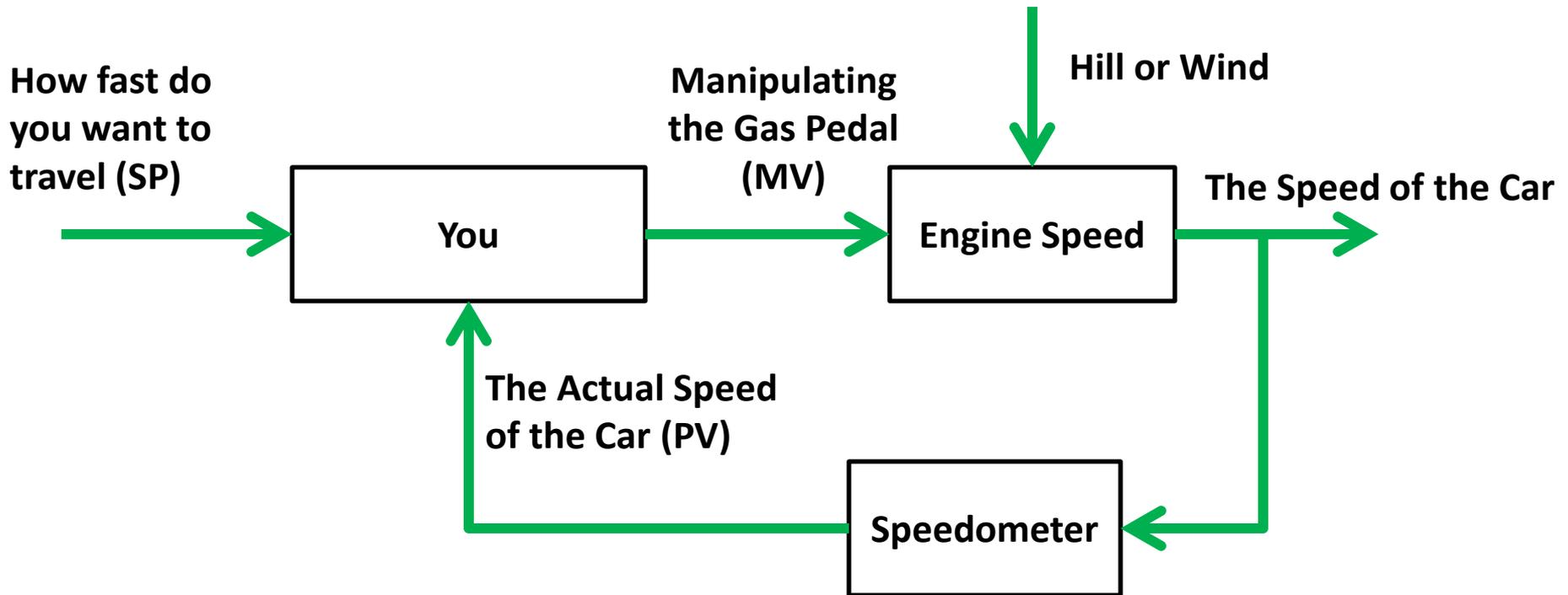
Classic block diagram of a PID Loop – Cruise Control
