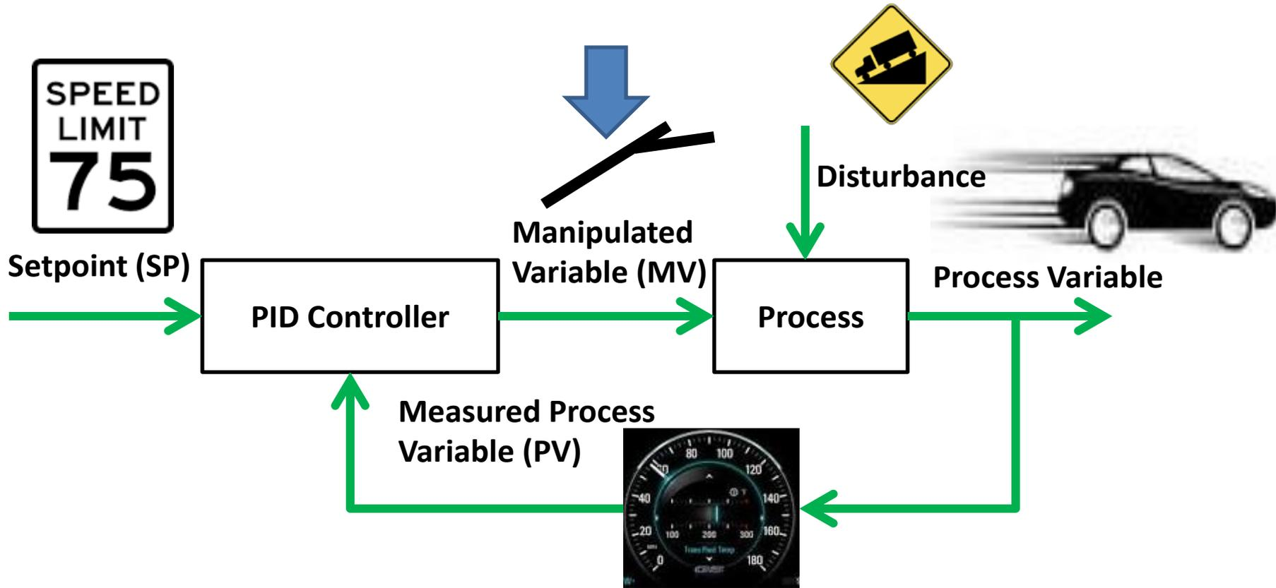
Block diagram of a Cruise Control PID Loop
