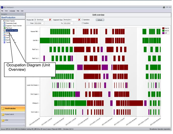
MES Beer Production allows an comprehensive overview per batch of e.g. alarms and exceptions, fermentation-graphs, confirmations to ERP as well as an overview of each unit in terms of CIP stats and / or fill-level.
