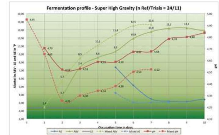
Figure 5. Fermentation profiles for Dynamic vs. Standard fermentation of VHGB beer (OE=24.5°P), showing the differences in extract, alcohol and pH trends
