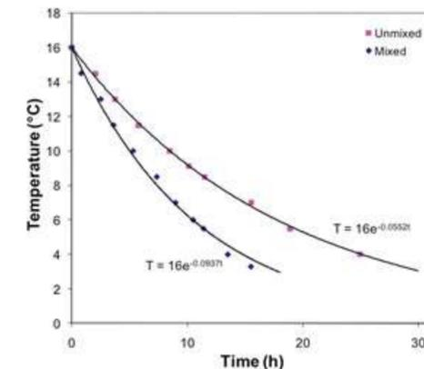
Figure 4. Effect of mixing on cooling time in an 1800 hL CCT.
